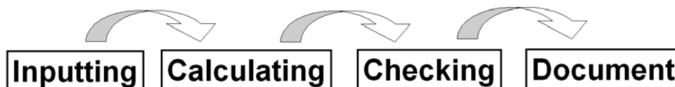
Figure 2 The stages of the calculation for a Scia Engineer project. In practise one adapts often the input during the checking phase.
